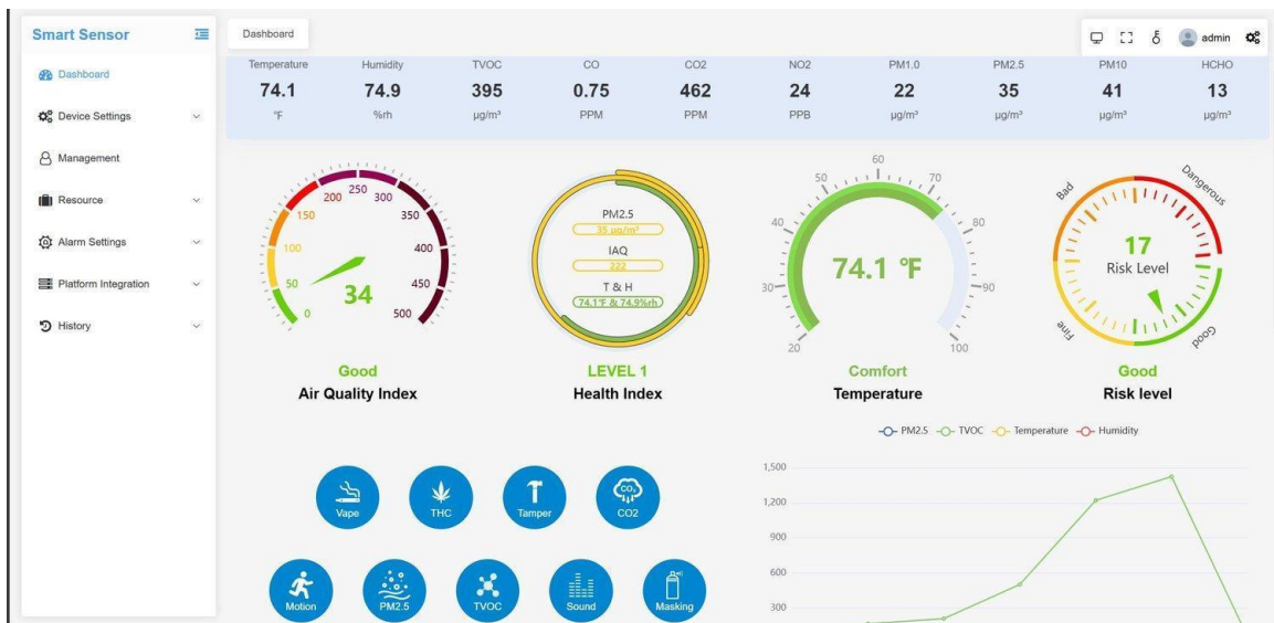
Figure 3-1. The live dashboard, presenting AQI, Health Index, temperature, risk level, and the individual sensor gauges.
