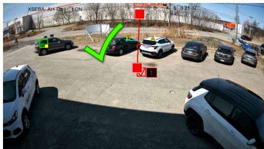
Figure 10-11. Example of crossing-direction rule configuration.
